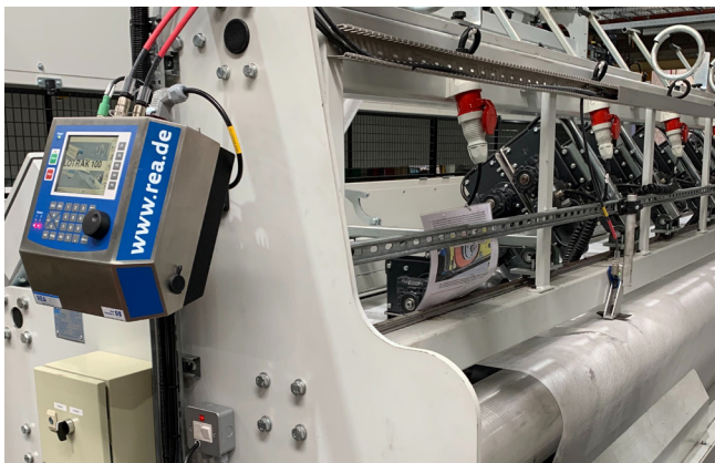
Marking of mesh material
